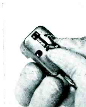
3 Insert new stylus into cartridge with fingers.
